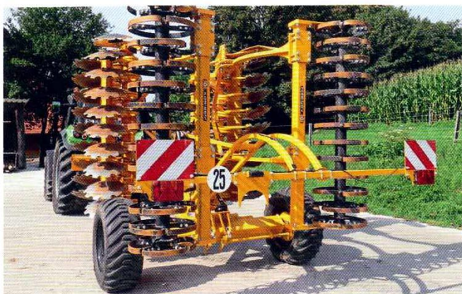
The folded 4.5m Disc-O-Mulch measures comfortably under 3m wide. The transport speed is set at 25km/hr max.
