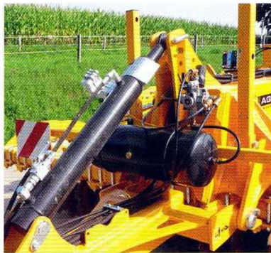
Where the front depth control ram is used, setting is by drop-in spacers.
