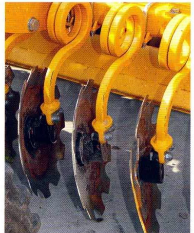
Big 35mm x 35mm pigtail legs carry the discs. With 215kg/leg, penetration wasn’t a problem.
