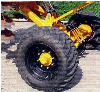
Tyres seem small for a 7.75t cultivator. There's plenty of room for bigger boots.
