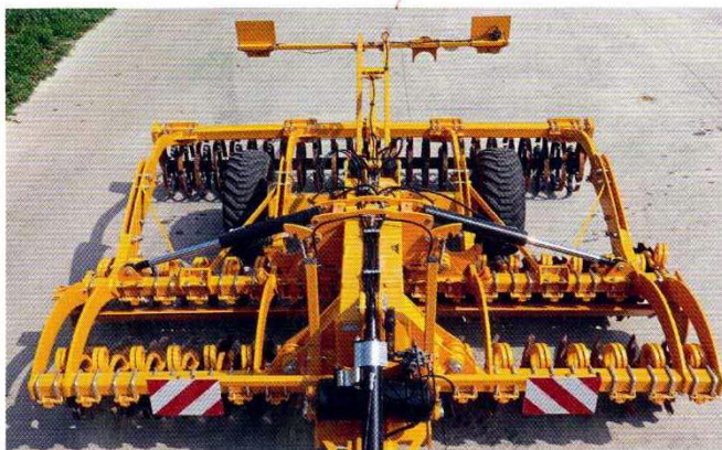
Lateral rams fold weighty wings up for transport. The spindly-looking lighting arms are now stronger.
