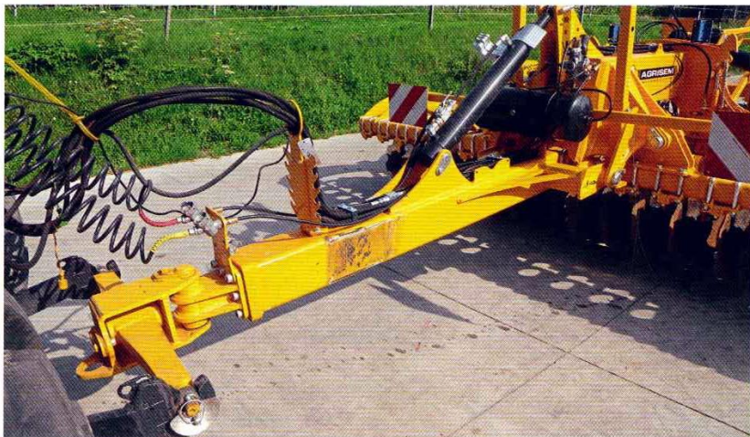
Attachment is by ball hitch or, as here, by linkage drawbar. The hose holders and cable routing could be better. When a ball hitch is specified, the ram (right) controls the front of the machine.
