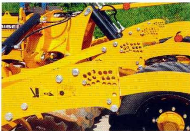
Four sets of pin-and-hole adjusters control working depth. Stickers show hole choice.
