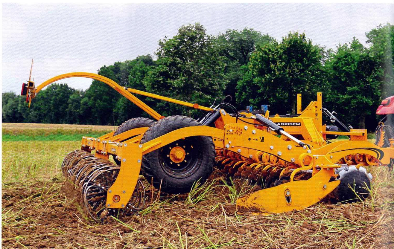
Agrisem's Disc-O-Mulch can be mounted or trailed; widths run from 3m to 12m. For part of the test we teamed the 4.5m version with a 120hp tractor.
