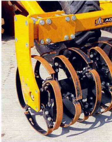
The Flexi-Roll press on the test machine used individual segments of 50mm wide steel, arranged in a spiral. One of eight roller options, it worked very well. Segment width has since been increased to 80mm.
